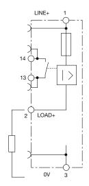
operating condition: 13-14 closed fault condition: 13-14 open
